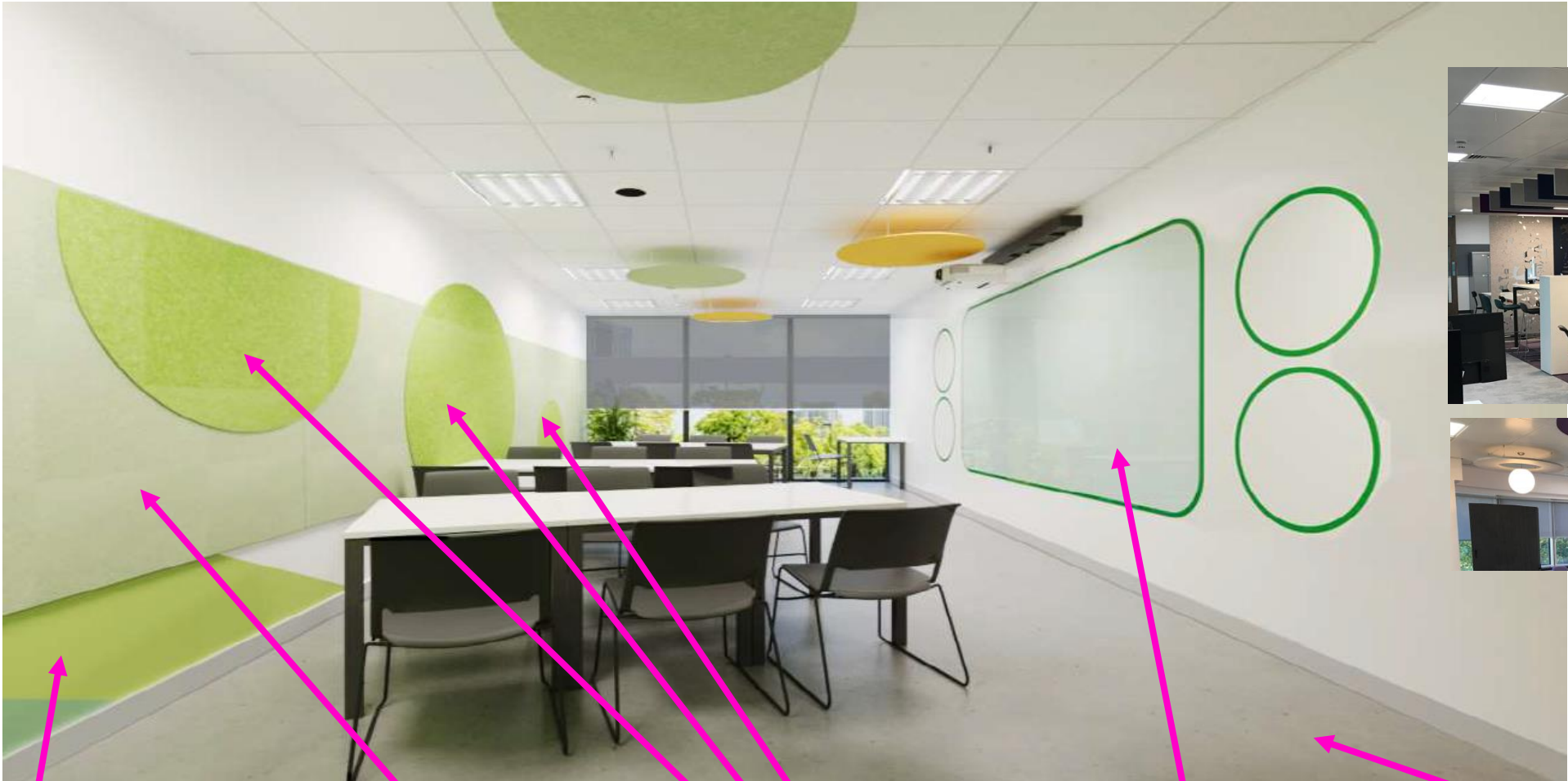
Raised cut out panels, if painted, can be removed easily for re-painting of wall, avoid placing these on same walls as pin boards
